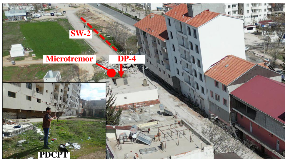
Figure 21. Locations of PDCPT, MASW and microtremor measurement conducted near buildings with subsidence / tilting damage ( 37^{\circ}47'26.57''\text{N} , 37^{\circ}39'7.88''\text{E} )
