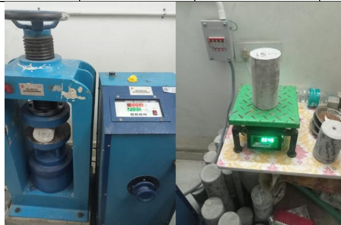
Figure 4. Testing of cylinder specimens for split tensile strength evaluation.
