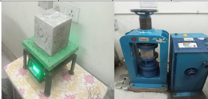
Figure 2. Moulding and testing of concrete specimens to determine compressive resistance
