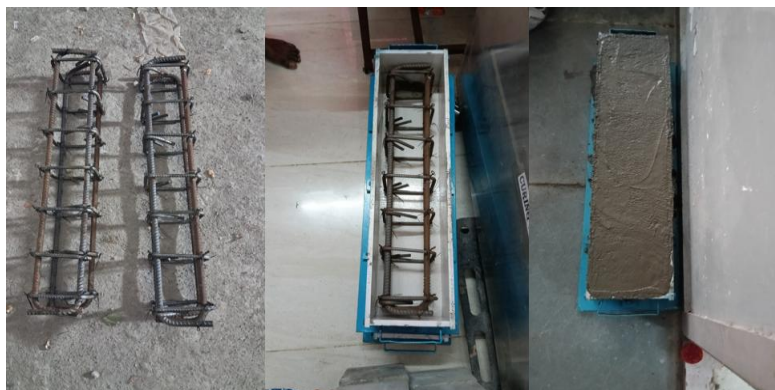
Figure 6. Casting process of RC beams with foundry sand replacement.
