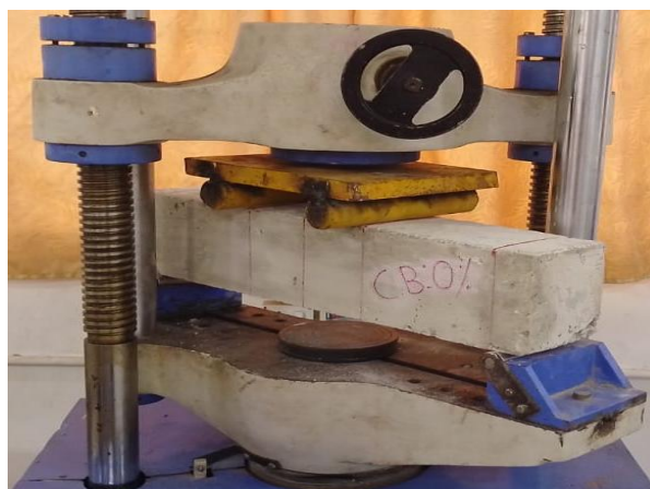
Figure 7. UTM was employed to examine the flexural strength of reinforced concrete beams.
