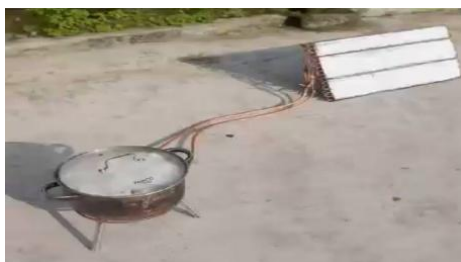
Figure 1. low-cost solar stove prototype utilizing recycled heat exchanger and pressurized air for sustainable cooking
