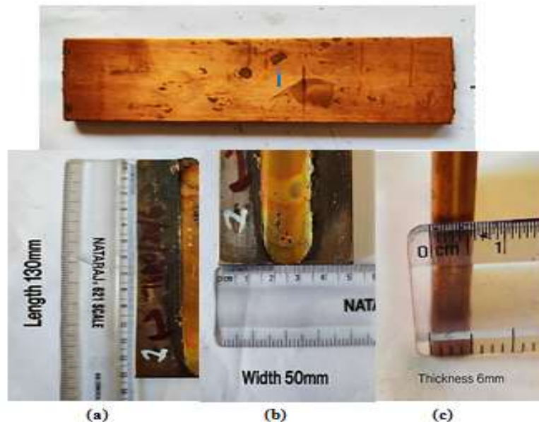
Figure 1. Dimensions of the commercial pure copper base plate used for friction stir processing
