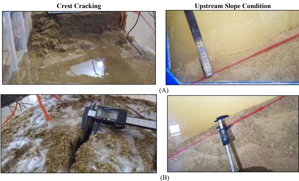
Figure 19. Maximum crest crack width
